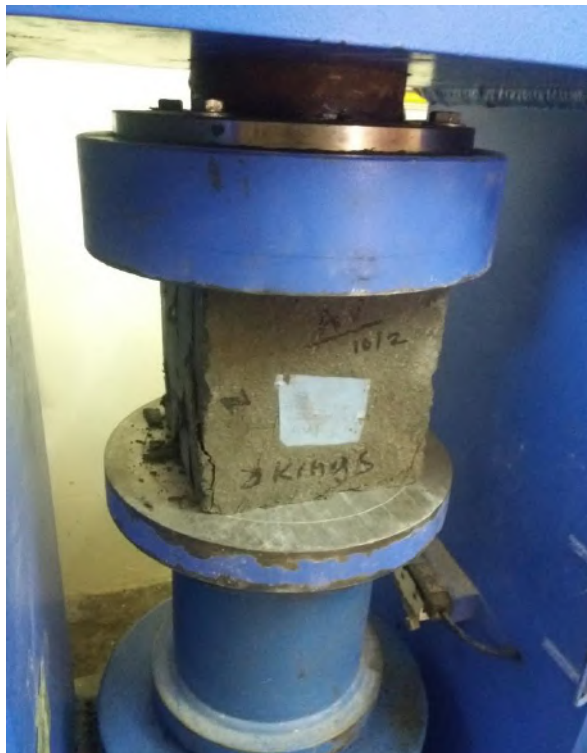
Fig.3.4: During Compression test of a cube in CTM
