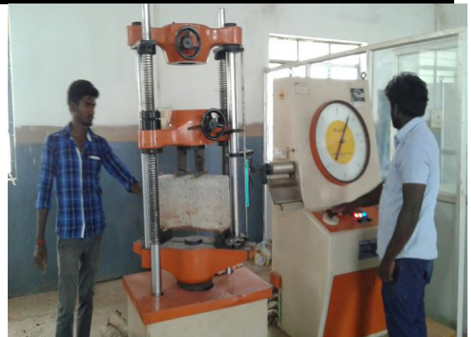
Fig.3.10: Flexure Test of a deep beam under third point loading in UTM of 400 kN capacity.
