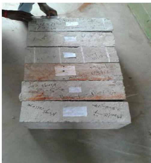
Fig.3.9: Marking on Deep Beams for third Point Loading with a chalk
