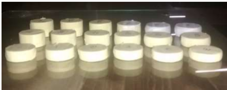
Fig. 3: Deformed Al-ZrB 2 composites of different aspect ratios covered with Teflon tape for density measurements.
