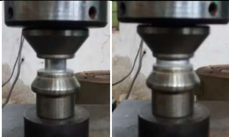
Fig. 2: Al composite before and after deformation between the flatens.
