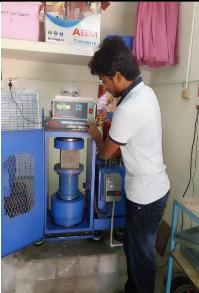
Fig.3.3: Placing the cube in CTM machine to check for design mix.
